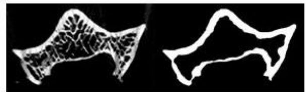
Figure 1: Micro-CT Image (left), Processed image with removed cancellous bone (right)
