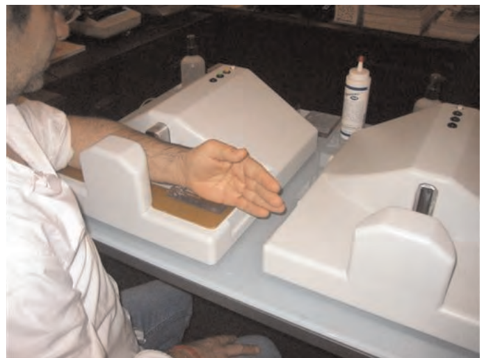
Fig. 1. UltraScan 650 device for measuring radial BMD.
